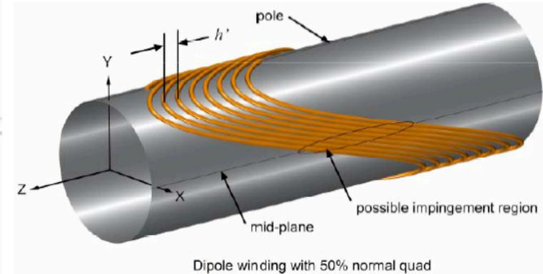
Figure 2. Dipole windings with 50% normal quad amplitude. The turn spacing,  $h'$ , has been increased due to the conductor impingement effect at the mid-plane.
